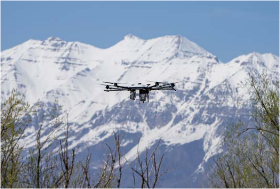
↑ Fortem Technologies The DroneHunter F700 can capture or disable an offending drone using its net guns and parachute. Captured drones can be towed to a specified location. ↓ Planet Under a contract with NASA, the company provides satellite data such as this image of the Athabasca Sand Dunes in Saskatchewan, Canada.
